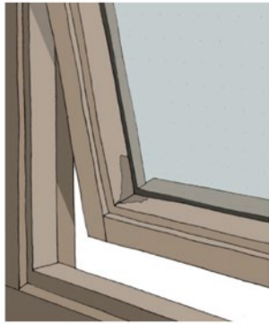
① Minor Repairs Small areas of degradation will be repaired using two-part resin to infill the damaged area.
